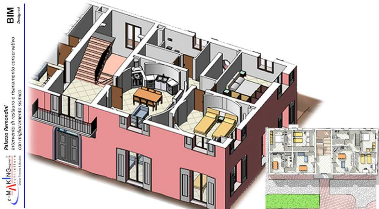
Fig. 14 – BIM modelling - preservation of the existing architectural layout.
